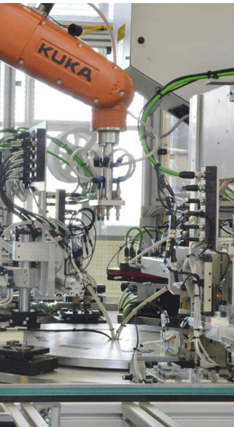
Rotary indexing machine for fully automated assembly of the pole and anchor plate.
